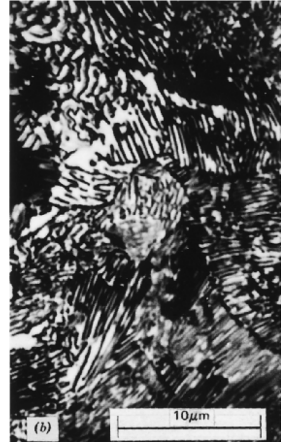
“Low” temp / fine spacing “fine pearlite”
